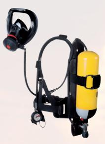
Our SCBA range includes self-contained open circuit breathing apparatuses with full face mask and demand valve, in compliance with EN 137. The **Advanced** and **Industrial** are Type 1, for general use, and also available in the Type 2 version, which positively passed the flash-over test.
